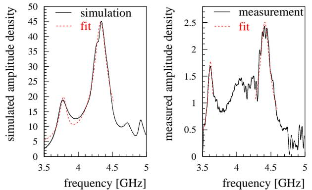
Figure 4: The spectrum of the signal from the damping waveguides after the transition as it was simulated with HFSS (left) and as it was measured (right).
