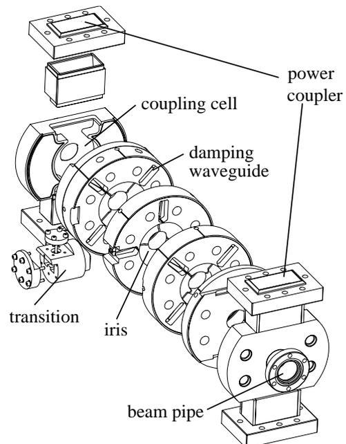
Figure 1: The SICA accelerating structure prototype.
