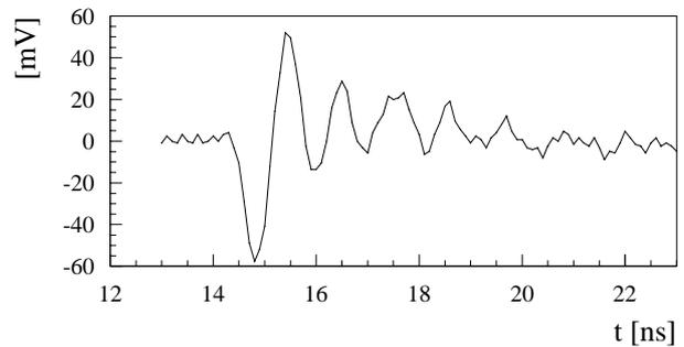
Figure 3: Measured time domain signal from the damping waveguide after mixing with a 3.498 GHz local oscillator.
