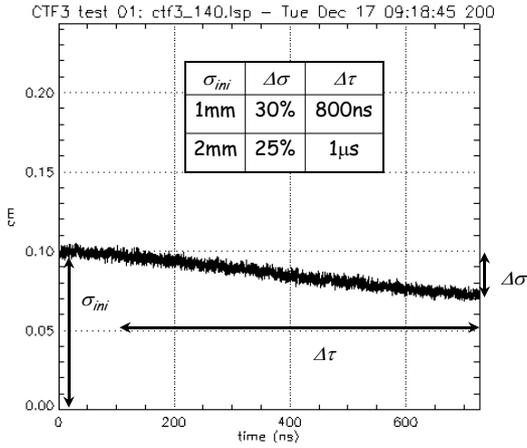
Figure 5: Time evolution of the R.M.S beam size
