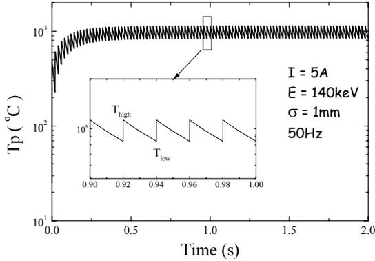
Figure 1: Graphite target temperature versus time
