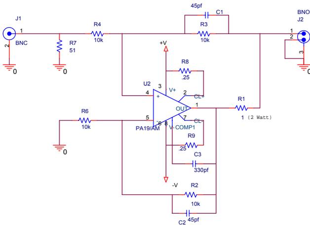
Figure 1: Breadboard of the Improved Howland Current Pump.
