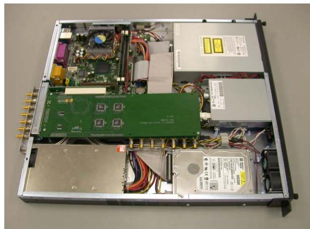
Figure 3. The SNS linac BPM system in a 1U, rack-mounted PC configuration.
