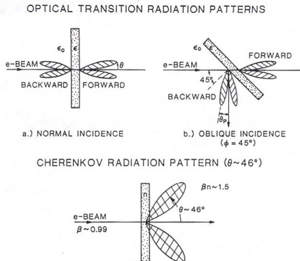
Figure 2: A schematic of the OTR radiation cases for normal incidence and for the foil at  $45^\circ$  to the beam direction. Backward and forward OTR are emitted at the two interfaces. The Cherenkov radiation pattern is shown for comparison.
