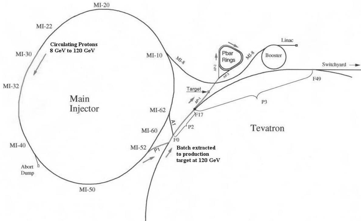
Figure 1: A schematic of the FNAL complex showing the linac, booster, Main Injector, Tevatron, and the transport lines between them.
