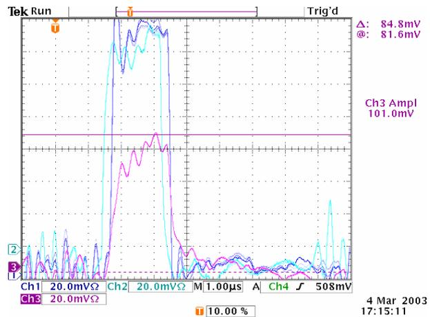
Figure 8: Peak currents at the polarized source, the chopper, and at the end of the linac. As seen there are no losses up to the chopper, and capture efficiency is 50%.
