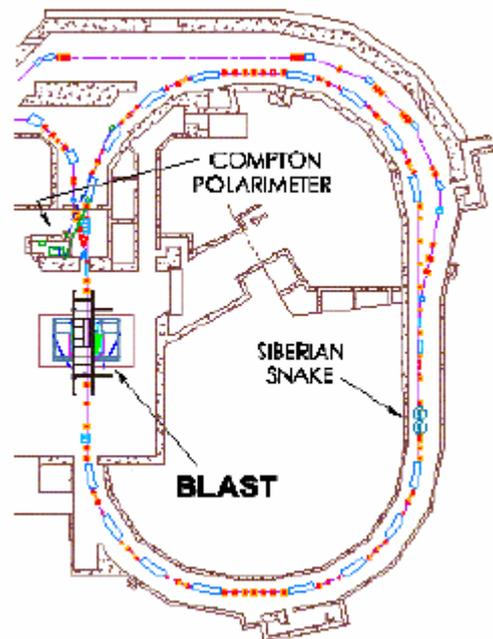
Figure 1: The Bates South Hall Ring with internal target area (BLAST)
