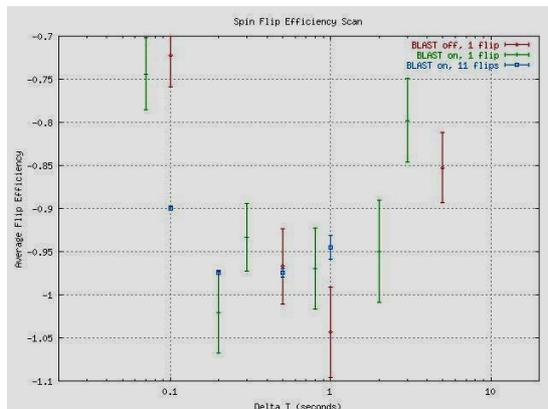
Figure 6: Polarization after a spin flip. Data are taken with and without the magnetic field from the BLAST toroid. The polarization of the data point with the smallest error bar was measured after 11 consecutive spin flips.
