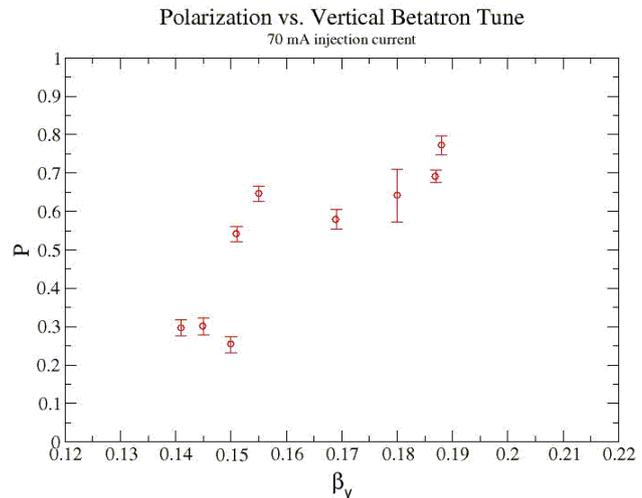
Figure 4: Measured beam polarization as a function of the vertical betatron tune.
