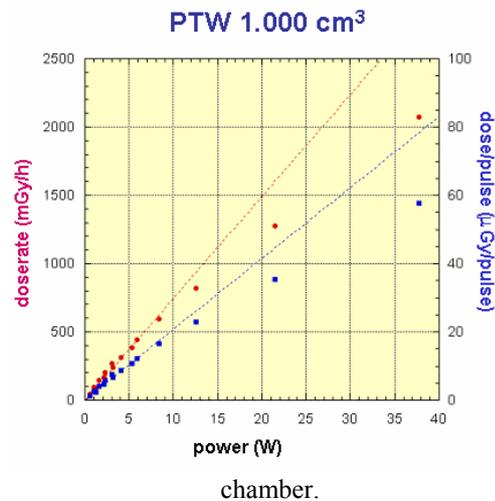
Figure 3b: Response of the 32002-PTW ionization chamber.
