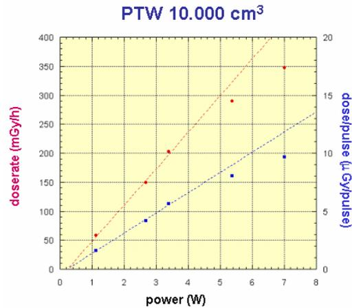
Figure 3a: Response of the 32003-PTW ionization chamber.
