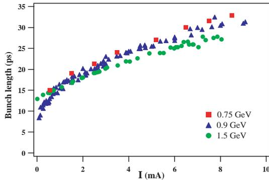
Figure 2: Bunch length as a function of the beam current (single bunch) at 0.75, 0.9 and 1.5 GeV. Data have been acquired by means of a double sweep streak camera. The absolute error on each point is about 2 ps.
