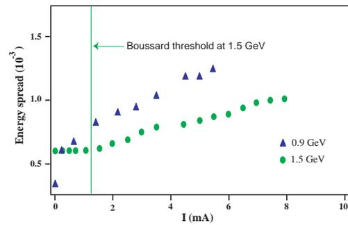
Figure 3: Beam energy spread as a function of the beam current (single bunch) at 0.9 and 1.5 GeV. The natural (i.e. close-to-zero current) values at 0.9 and 1.5 GeV are  $0.36 \cdot 10^{-3}$  and  $0.6 \cdot 10^{-3}$ , respectively.
