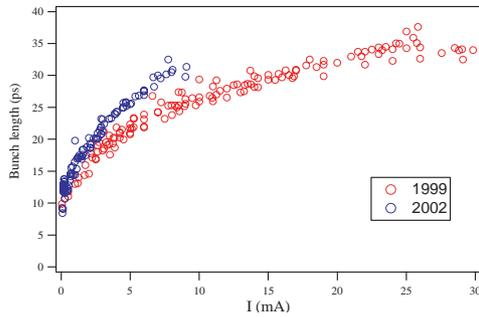
Figure 1: Bunch length as a function of the beam current (single bunch). Measurements performed in 1999 and 2002 at 0.9 GeV. Data have been acquired over the whole current range by means of a double sweep streak camera. The absolute error on each point is about 2 ps.
