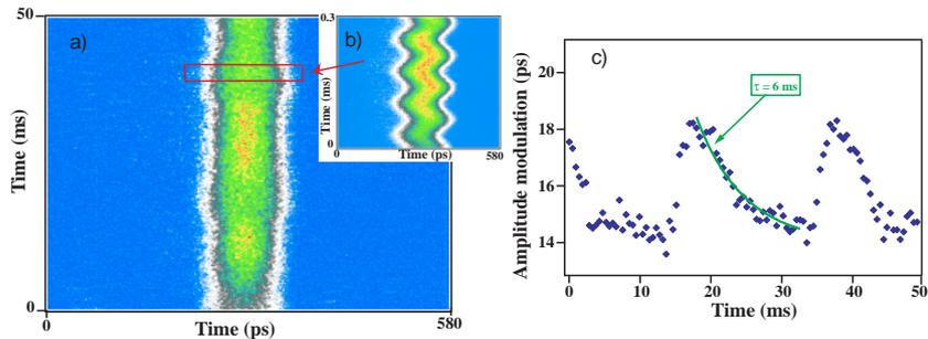
Figure 5: Figure a): streak camera image of the electron beam at 0.9 GeV (6 mA). Figure b): Evolution of the position of the beam center of mass of as obtained by the analysis of Figure a).
