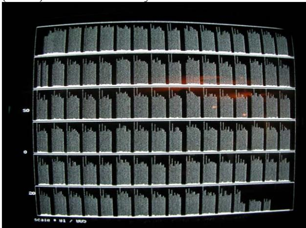
Figure 1: Luminosity per bunch for typical by-3 pattern.
