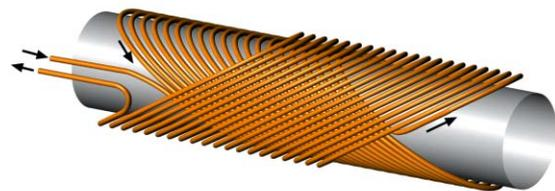
**Figure 2:** Double helix dipole (DHD) concept uses pairs of layers with opposite tilt and current direction. Aperture may be circular or elliptical. High field values can be obtained by using multiple pairs of layers with the transition between layers as shown.
