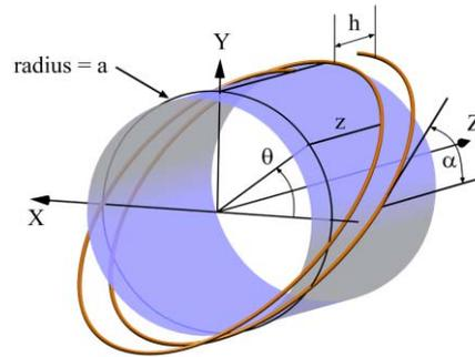
**Figure 1:** For the case of the dipole, the  $z$  coordinate of the conductor path is given by  $z = h + A_0 \sin\theta$  with  $A_0 = a / \tan\alpha$ , where  $a$  is the radius of the coil aperture,  $\alpha$  is the tilt angle of the winding with respect to the horizontal axis, and  $h$  is the helical advance per turn.
