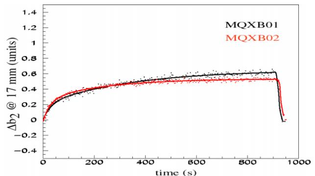
Figure 3: Decay and snap-back of the dodecapole component for a plateau at injection of 15 min.
