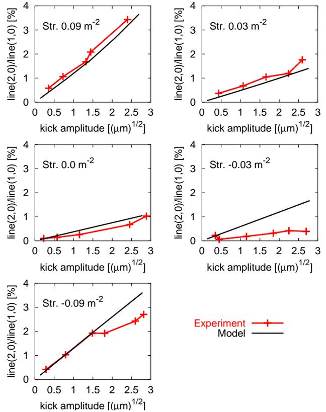
Figure 3: Measurement of the first order resonance. The normalised amplitude of the spectral line (2,0) is plotted versus horizontal betatron amplitude for five different strengths of the sextupole. Experimental results are multiplied by the decoherence factor of 2 and predictions from the model are shown.
