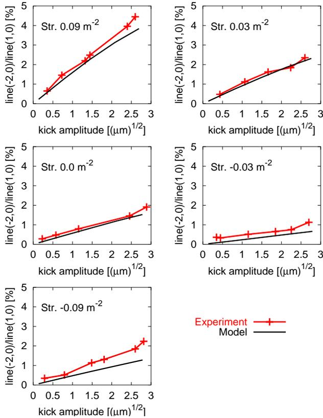
Figure 2: Measurement of the third order resonance. The normalised amplitude of the spectral line (-2,0) is plotted versus horizontal betatron amplitude for five different strengths of the sextupole. Experimental results are multiplied by the decoherence factor of 2 and predictions from the model are shown.
