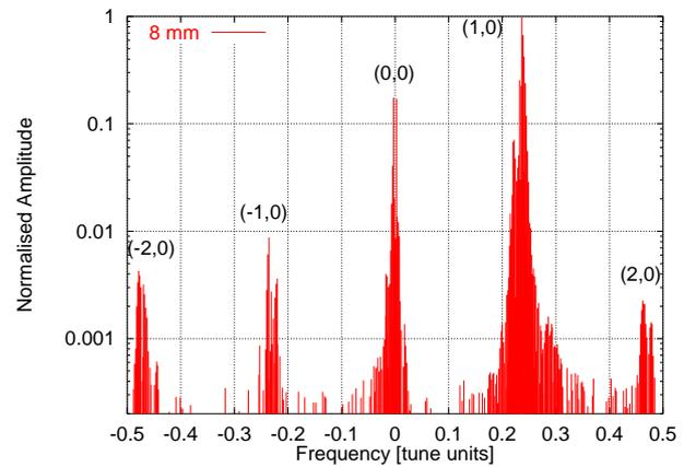
Figure 1: Fourier spectrum of the complex signal from pick-ups *yo5-bh10* and *yo5-bh12* for the unchanged RHIC and for an oscillation amplitude of 8 mm. The label  $(m,n)$  means that the frequency is equal to  $m\nu_x + n\nu_y$ .
