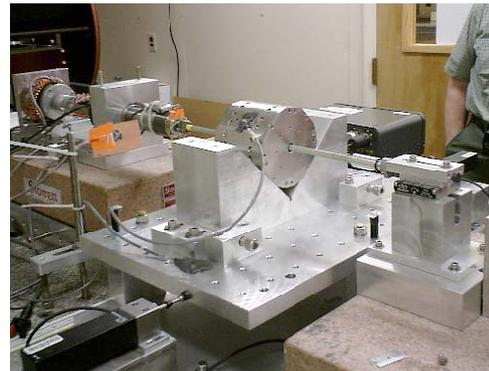
Fig. 8 Magnetic field measurement setup at SLAC.
