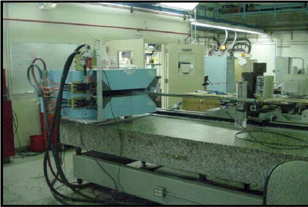
Figure 1. GX Dipole on Stepper Stand
