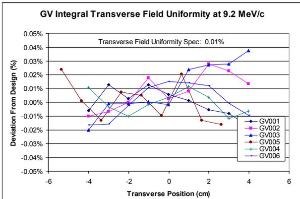
Figure 2. GV Integral Transverse Uniformity
