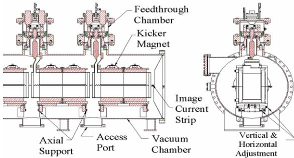
Figure 4. Cross Section Of Kicker Assembly
