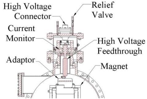
Figure 5. Feedthrough Chamber
