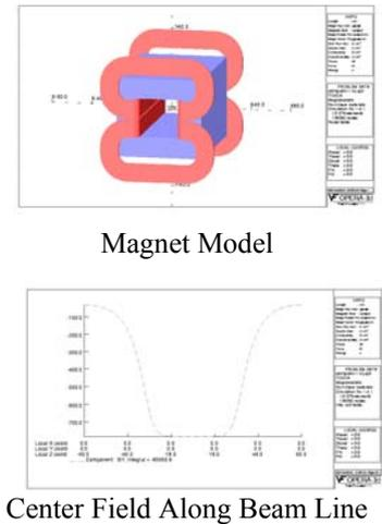
Figure 6: Magnetic Field Plot
