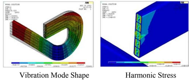
Figure 8: Harmonic Analysis of Coil
