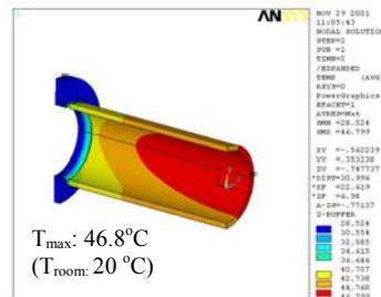
Figure 5: Eddy Current Heating In The Chamber
