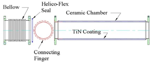
Figure 4: Vacuum Chamber Components
