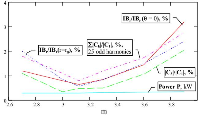
Figure 2. Octupole magnet parameters versus the order of tip shape  $m$  at fixed magnet parameters  $2.56\text{T/m}^2$ ,  $\Delta\theta=38.6^\circ$  (no clamps),  $r_g=12.5\text{cm}$ , and magnetic aperture radius  $r_{ap}=150\text{mm}$ .
