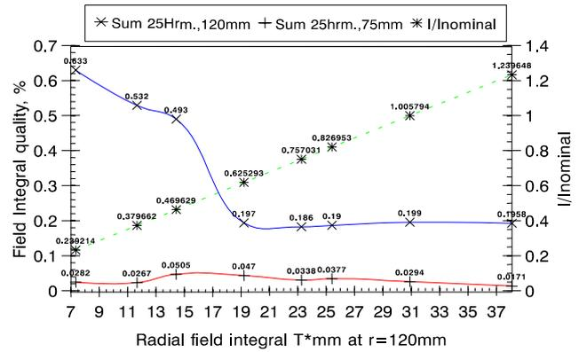
Fig. 4. Normalized sextupole field integral  $I/I_{nominal}$  (right ordinate axis) and its quality  $\sum|C_k|/|C_1|$  for 25 unwanted harmonics (on the left axis) vs field integral at  $r_g=120mm$  and  $r_g=75mm$ . Parameters:  $P_{max}=2.8kW$ ,  $m=2.671$ ,  $r_{ap}=150mm$ , pole tip angle  $\Delta\theta=44.9^\circ$ .
