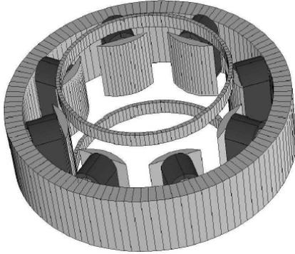
Figure 1. Magnetic design of a short octupole with ring field clamps, cylindrically shaped pole tip and standard racetrack coils.
