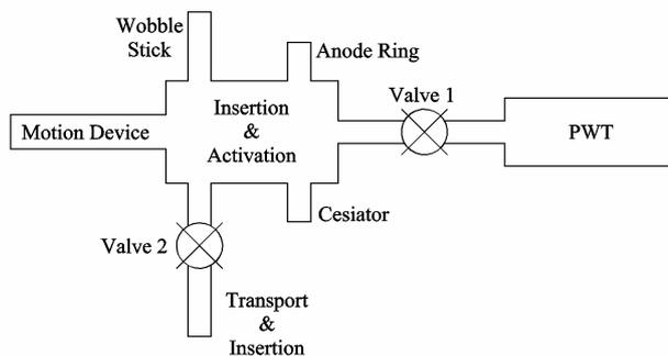
Figure 4: Block diagram of the load lock system.
