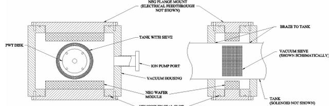
Figure 2: Schematic showing the circumferential sieve layout including the NEG modules and vacuum housing.
