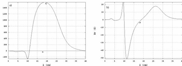
Figure 7: a) Axial and b) radial magnetic fields in the new PWT solenoid magnets. The radial field is taken near the edge of the electron beam envelope. The cathode plane is at  $z = 10.92$  cm, where the axial field is null.
