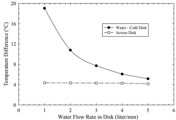
Figure 8: Temperature difference for the PWT disk as a function of flow rate. Solid line: temperature difference between the water and the coldest point on the disk; dashed line: thermal gradient across the disk.
