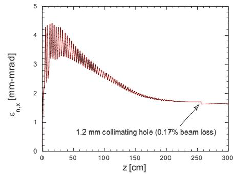
Figure 2: PARMELA results for the evolution of the transverse normalized rms emittance in hybrid injector. Effects of collimation (1.2 mm radius tube) of beam edge shown.
