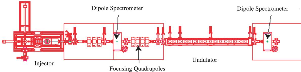
Figure 1: CAD Drawing of the PEGASUS Beamline.
