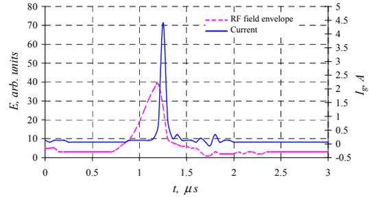
Fig. 4: RF field envelope in the gun cavity and the beam current at the gun output
