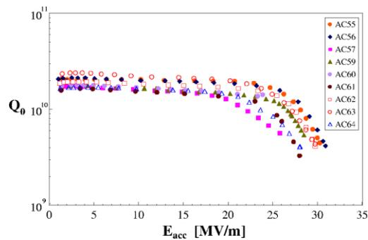
Figure 5: Vertical dewar results for cavities from the 3rd production processed with BCP [2].
