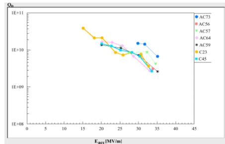
Figure 6: Horizontal pulsed test results of TESLA cavities. AC73 is electropolished, the rest have BCP treatment.
