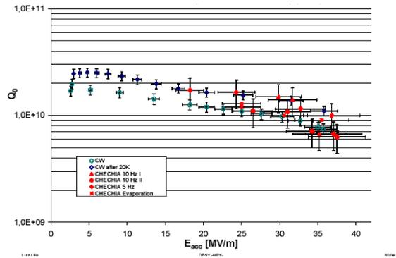
Figure 8: Horizontal pulsed test of EP cavity AC73.
