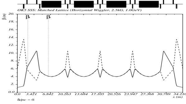
Figure 1: Dispersion-free OK5 FEL lattice at 1 GeV. Powered as horizontal wigglers, the maximum field in the OK5 is 2.5 KGs. The solid and dashed lines are  $\beta_x$  and  $\beta_y$  respectively. At the center of the wiggler,  $\beta_x = \beta_y = 4$  m.
