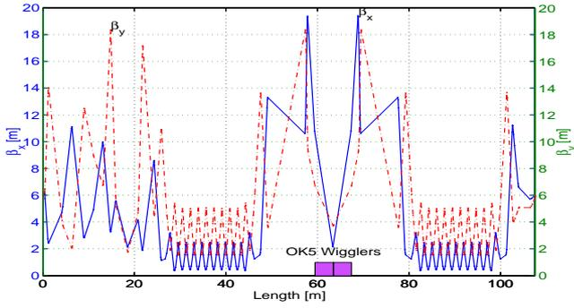
Figure 2:  $\beta$ -functions for the Duke ring with two OK5 wigglers located at the center of the FEL straight ( $\beta_x = 2.14$ ,  $\beta_y = 3.75$  m). The beam energy is 300 MeV and OK5 wigglers are circularly polarized with a peak field of 1.8 kG for each wiggler array. The solid and dashed lines are  $\beta_x$  and  $\beta_y$  respectively.
