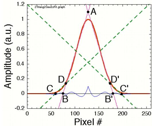
Figure 3: result of the bi-triangular fit to a test Gaussian profile. The fit to the core is represented by the dotted purple lines (area  $ABB'$ ), while the fit to the halo is represented by the dashed green line (area  $BCD$  and  $B'C'D'$ ). The thin blue line is the difference between the fit and the Gaussian curve.
