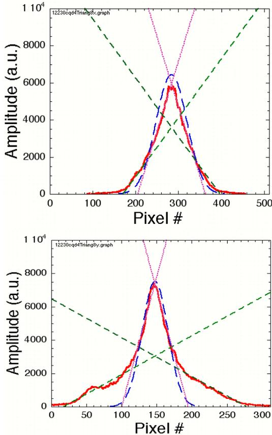
Figure 5: The  $x$  (top) and  $y$  (bottom) beam profiles (red lines) from the beam on Fig. 2, and their fits: Gaussian (blue line), and bi-triangular core (purple dotted lines) and halo (green dashed lines). The halo is larger in the  $y$ -profile.
