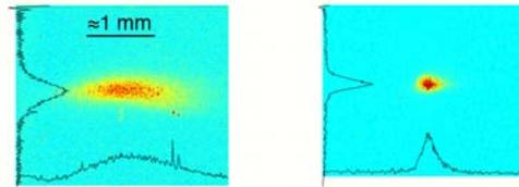
Figure 1: OTR images of the electron bunch without plasma ( $n_e = 0$  left), and with  $n_e \approx 10^{14}$  cm<sup>-3</sup> (right) with the  $x$  (horizontal) and  $y$  (vertical) beam profiles. Without plasma the beam size is asymmetric because the beam emittances are different in the  $x$  and  $y$  planes.
