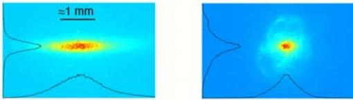
Figure 2: OTR images of the positron bunch without plasma ( $n_e=0$ , left), and with  $n_e\approx 10^{14}\text{ cm}^{-3}$  (right) with the  $x$  (horizontal) and  $y$  (vertical) beam profiles. Without plasma the beam size is asymmetric because the beam emittances are different in the  $x$  and  $y$  planes.
