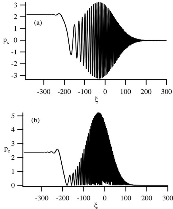
Figure 2 Dynamics of an electron interacting with a chirped pulse,  $\mathbf{p}_0=0$ ,  $a_0=3$ ,  $\sigma=100$ , and  $\Delta\Omega=0.51$ .
