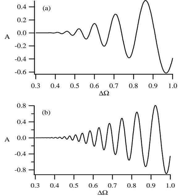
Figure 1: Electron's transverse momentum gain  $A$  after interaction with a chirped EM pulse,  $a_0=0.1$ ,  $\sigma=50$  (a) and  $\sigma=100$  (b).
