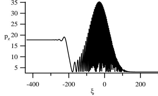
Figure 3: The calculated longitudinal momentum of an electron. All parameters are the same as those in Fig. 2 excepting initial longitudinal momentum,  $p_{z0}=3$ .
