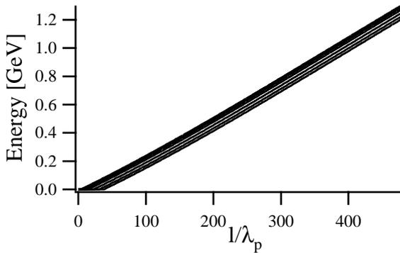
Figure 4. Energy of accelerating electrons,  $p_0=1$ ,  $L_0=10\lambda_p$ .
