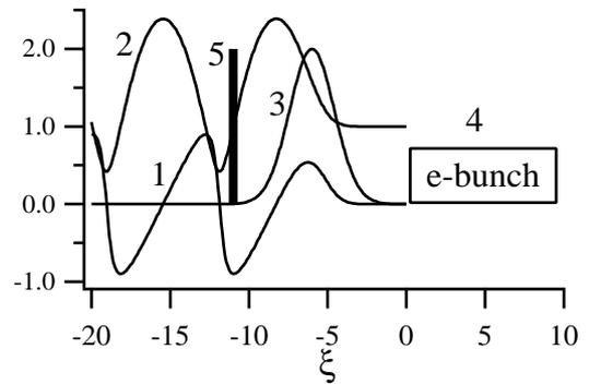
Figure 1: The laser wakefield scheme: the wake electric field  $E_z$  (1), the potential  $\Phi$  (2), the laser pulse amplitude  $a$  (3), the initial (4) and trapped (5) bunches as a function of the position in a moving frame.  $a_0=2$ ,  $\sigma_z=2$ ,  $\gamma_g=50$ .
