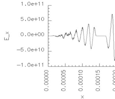
Figure 3: Longitudinal Electric field as a function of distance of propagation right before collision takes place. Notice the fast decay of the plasma wake field due to the channel.
