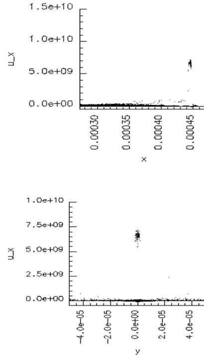
Figure 5: (a) Snapshot of electrons in  $X - V_x$  phase-space. (b) Snapshot of electrons in  $Y - V_x$  phase-space after about one Rayleigh length of propagation.
