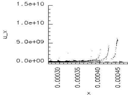
Figure 1: Particles in  $x - v_x$  phase-space phase-kick injection. We observed that a train of beamlets is formed.
