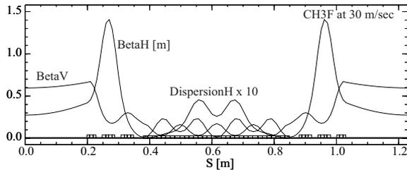
Figure 4: Beta and Dispersion of the CH<sub>3</sub>F Ring
