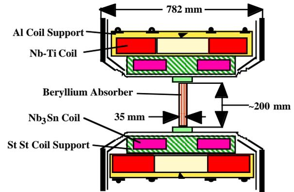
Figure 2. A Cross-section of the MICE Focusing Magnet with a Nb<sub>3</sub>Sn Insert Coil and a Beryllium Absorber
