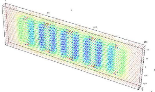
Figure 4 (Color): Vectorial representation of the fields in the gap of 11-pole gradient wiggler inside the 3D volume  $\{x=0-150; y=\pm 3; z=\pm 24\}$  cm. Medial plane of the wiggler  $\{x, z\}$  runs at  $y=0$ .
