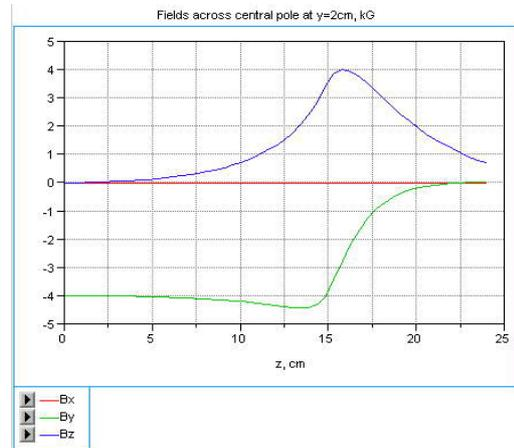
Figure 6 (Color): Fields across central pole, starting from  $z=0$ ,  $y=2$  cm. Material of yoke St1010. Points at  $\{x=75, y=2, z=0-24\}$  cm.
