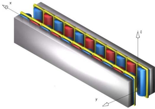
Figure 2 (Color): View to the gradient wiggler model.
