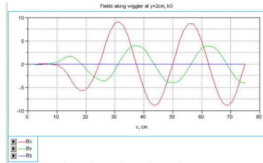
Figure 5 (Color): Field graphs for  $y=+2$  cm,  $z=0$ . Half wiggler is shown as in Figure 3. Center is at the right side of the plot at 75 cm.  $B_y$  comes to it's maximum,  $B_x$ , indeed comes to zero. Basically  $B_z=0$  along this axis as it must be according to symmetry properties.
