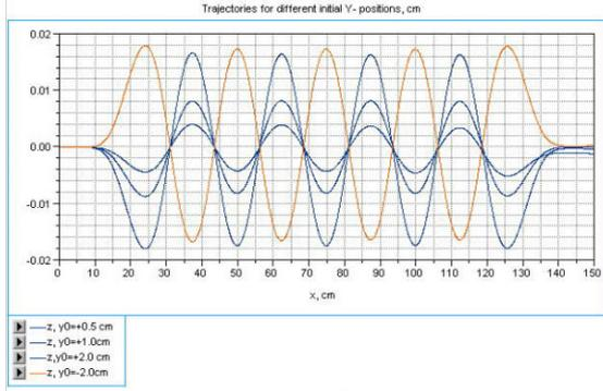
Figure 7 (Color): Trajectories for different initial positions in Y direction. There are shown ones for  $y_0 = +0.5$  cm,  $+1.0$  cm,  $+2.0$  cm,  $-2.0$  cm. The last one corresponds the start point below median plane. Beam energy 2 GeV.
