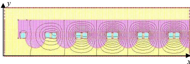
Figure 3 (Color): Lines of magnetic field in central plane of wiggler,  $z=0$ . Half of the wiggler is shown; right side of the plot is a plane of symmetry along  $x$ . Radiuses of the poles are 4 cm, period -25 cm. Gap between coils 0.5 cm. Length of the pole in  $z$  direction is  $\pm 15$  cm. Particles are moving from the left side.  $\{xz, y=0\}$  represents medial plane.
