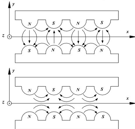
Figure 1: Dipole wiggler, upper one and gradient undulator/wiggler, lower. Beam is moving along  $x$ -axis. Normal to the drawing's plane is  $z$ -direction.
