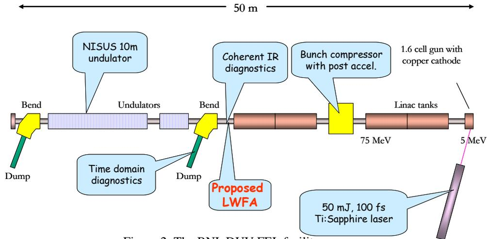
Figure 2: The BNL DUV-FEL facility
