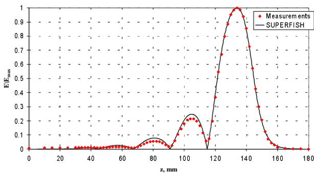
Figure 1: Distribution of on-axis field amplitude: calculated and measured.
