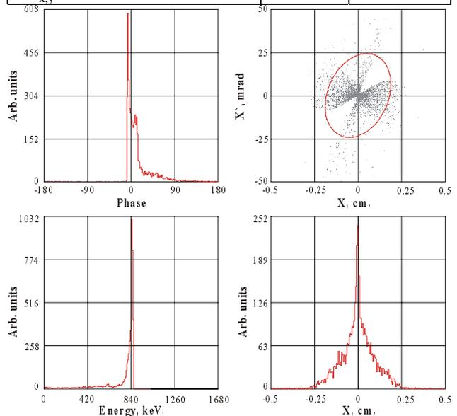
Figure 3: Beam characteristic on an exit of the buncher.
