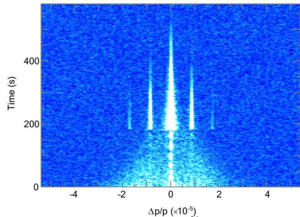
Fig. 2. Schottky spectrum of a  $\text{Xe}^{36+}$  beam with an rf voltage of 6 mV indicating the observed transition to an ordered state with a bunched beam.
