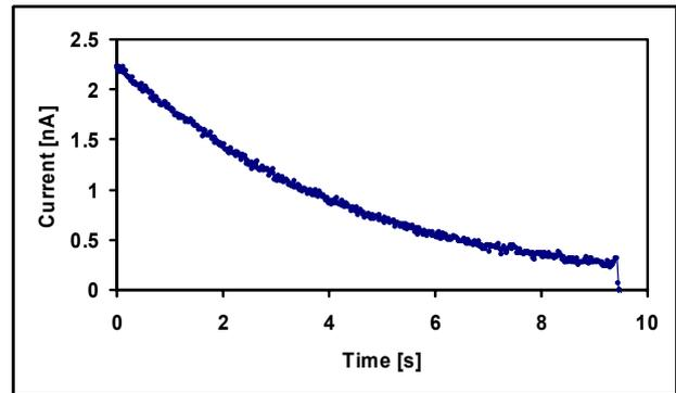
Figure 1: Current of a stored  $H_2S^+$  beam.
