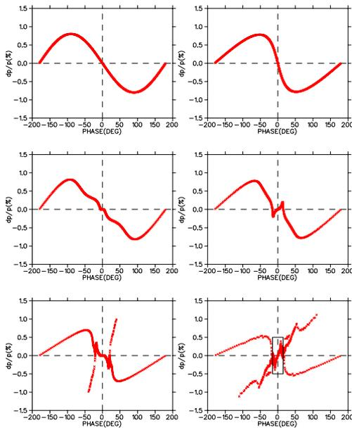
Figure 4: Simulated evolution of particle distribution in longitudinal phase space at  $600 \mu\text{A}$ . From left to right and up to down, windows respectively correspond to the following locations in Fig.3: (1)  $z=603$  inch; (2)  $z=781$  inch; (3)  $z=902$  inch; (4)  $z=1035$  inch; (5)  $z=1198$  inch and (6)  $z=1430$  inch. Of the 500 particles, 240 are lying inside the  $\pm 18^\circ$  phase window in the end.
