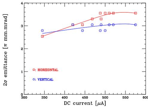
Figure 2: Fitted beam emittance ( $2\sigma$ ) vs. current.
