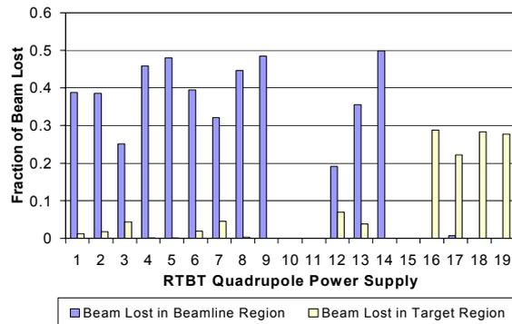
Figure 2: Fraction of beam lost in RTBT at the power supply setting which produces an off-normal “beam-in-footprint” condition.
