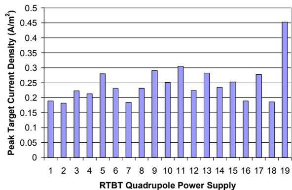
Figure 3: Peak current density achievable by tuning each power supply individually, leaving the others at nominal strength.
