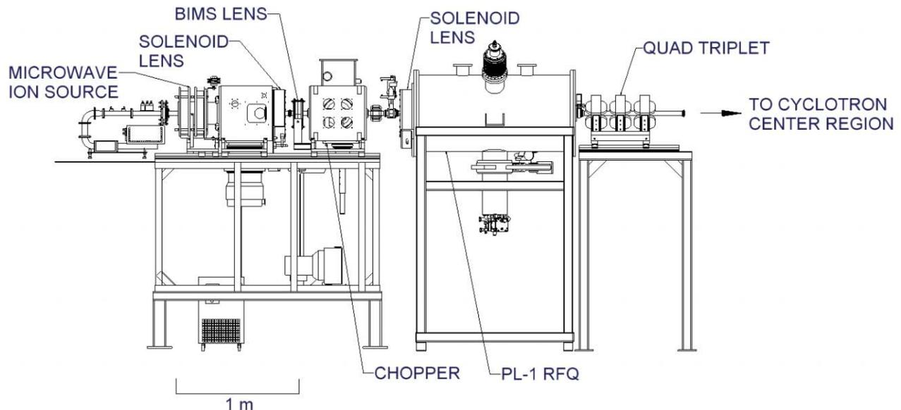
Figure 1: Schematic of the 750 keV proton injector. The beam height and centerline of the injector is 196.4 cm above the floor.
