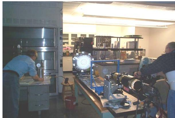
Figure 1: Photogrammetry setup for window tests..
