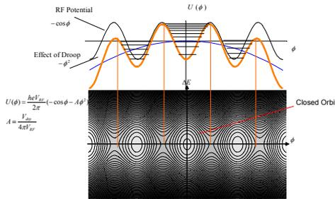
Figure 5: Effect of Voltage Droop in Potential Well
