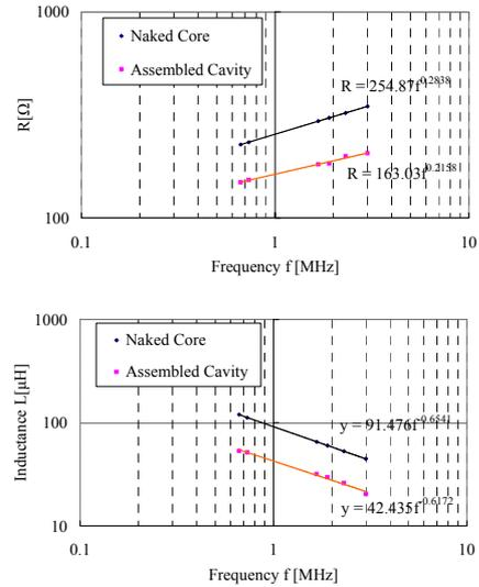
Figure 4: Comparison of Naked Core and Cavity
