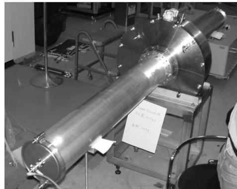
Figure 2: Induction Cavity with Transmission Lines
