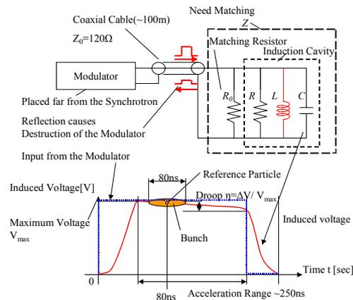
Figure 1: Induction Acceleration Setup
