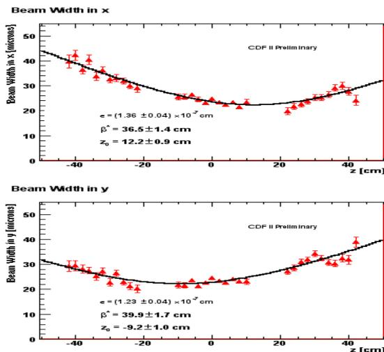
Figure 1 Example plot for one run of 20 runs showing luminous region size versus  $z$  and the fits to Equation 2. Typical correlation coefficients of the fits are about -0.8 for  $(\beta^*, \epsilon)$ , 0.5 for  $(\beta^*, z_0)$ , and -0.6 for  $(\epsilon, z_0)$
