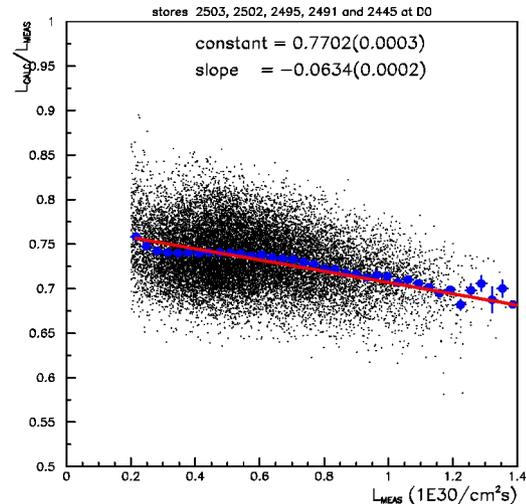
Figure 3 Ratio of calculated to measured D0 bunch-by-bunch luminosity during 5 stores versus D0 measured luminosity.
