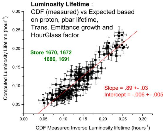
Figure 1: Correlation plot showing the predicted (based on various emittance and intensity detectors) vs measured luminosity lifetime. One data point corresponds to one  $p\bar{p}$  bunch in a given store. This data was taken during August 2002. Similar results have been obtained on recent stores.
