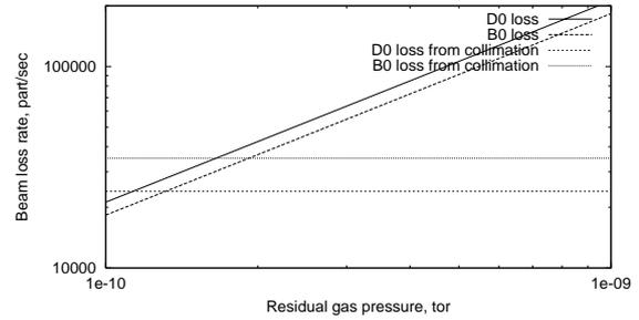
Figure 2: Beam loss rate upstream of D $\emptyset$  and B $\emptyset$  as a function of an average gas pressure. Also shown are beam losses upstream of D $\emptyset$  and B $\emptyset$  originated by the collimation system.
