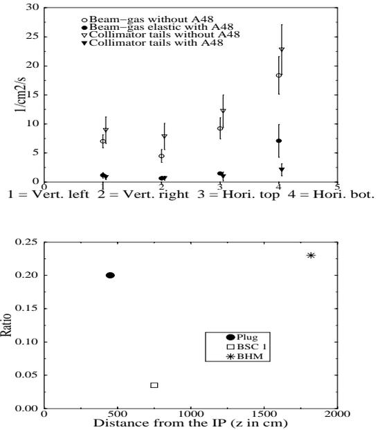
Figure 5: CDF BHM hit rate (top) and the main detector absorbed dose ratio with/without shadow collimator as a function of a distance from the IP (bottom).
