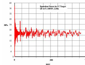
**Figure 4:** Beam-induced von Mises stresses on target
