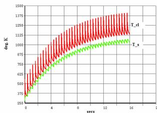
**Figure 3:** Transient temperatures in the C-C target
