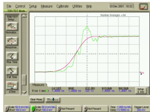
Figure 5. The risetime of a complete assembly is 1.5 ns, including the interconnections and vacuum feedthrough connectors. Data are in green, a 2-ns risetime filter in red.
