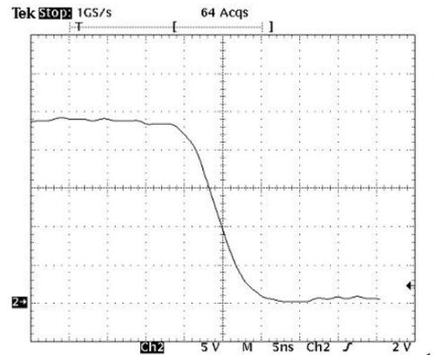
Figure 9. Expansion of trailing edge of typical output pulse showing fall-time of about 8 ns at 2350 volts
