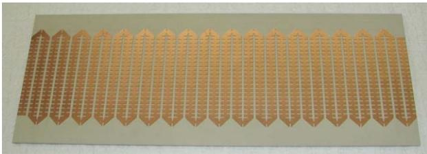
Figure 3. Etched circuit board prior to machining
