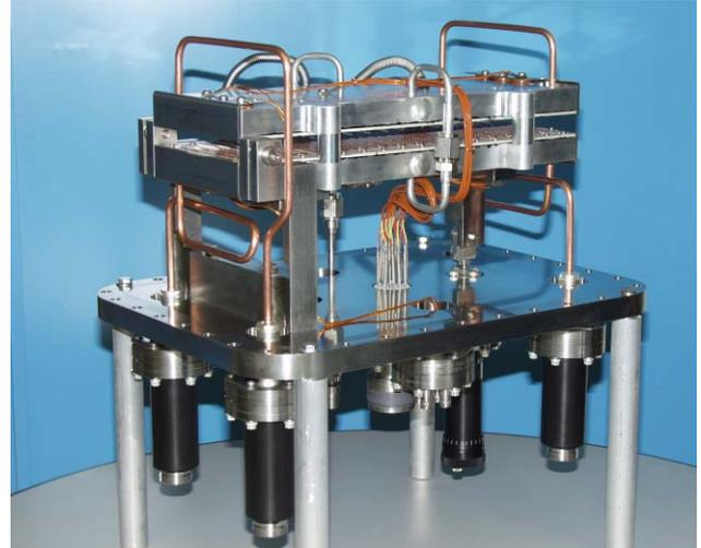
Figure 1. One of two completed MEBT-chopper structure assemblies. The unit is upside down from the normal mounting position on the beamline.
