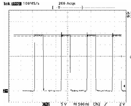
Figure 8. String of four pulses (out of ~1000 during a 1-ms SNS macropulse)
