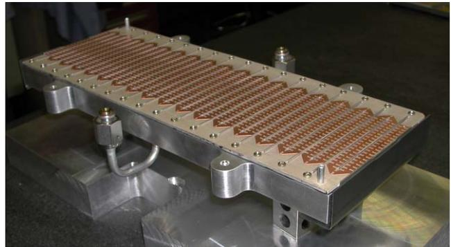
Figure 4. Finished circuit board glued to ground plane
