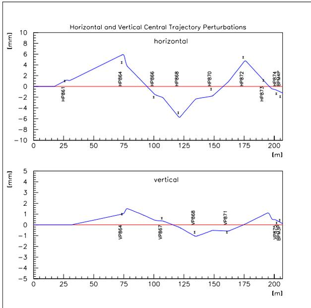
Figure 2. Example horizontal and vertical dipole changes
