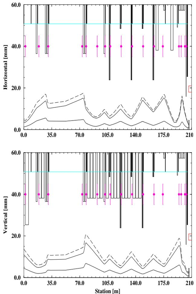
Figure 1. Beam envelope and apertures. The lower beam envelope is the one sigma and the two upper traces are the 95% and 99% with momentum folded in. The assumed emittances were 20 PI and a  $dp/p$  of .1%. The line indicates the total loss monitor coverage and the dots indicate the location of individual loss monitors.
