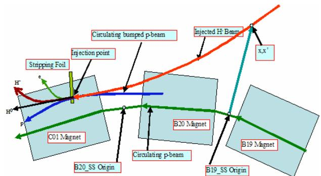
Figure 2. Schematic diagram of injection region in AGS.
