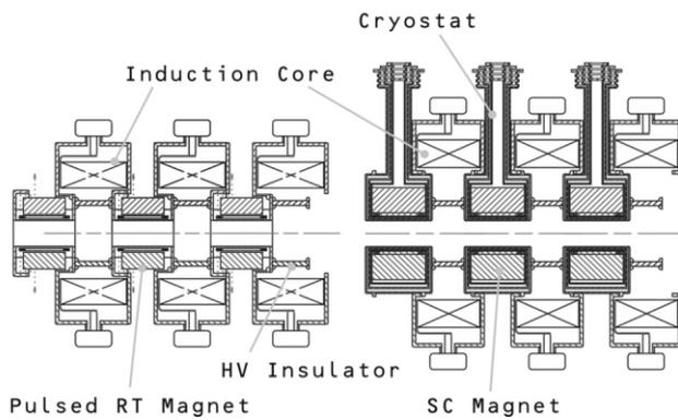
Figure 3: Comparison between a room-temperature (RT) version and a superconducting version (SC) of IBX. The cryostat for the SC case takes up additional radial space, leading to larger induction cores.
