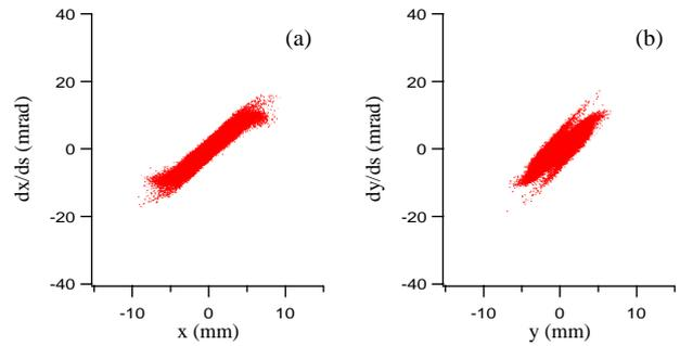
Figure 4: Phase-space distribution at the emittance monitor obtained with an IMPACT simulation for Measurement I. (a) Horizontal phase-plane. (b) Vertical phase-plane.
