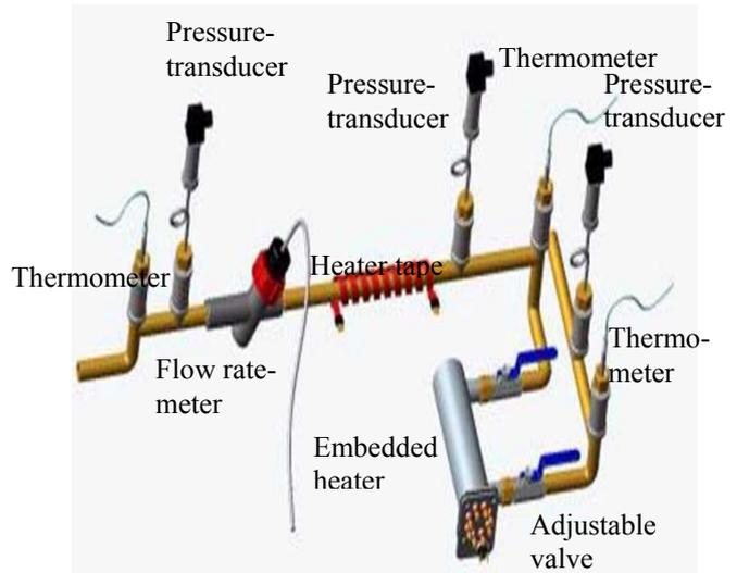
Figure 2: High precision temperature control experiment
