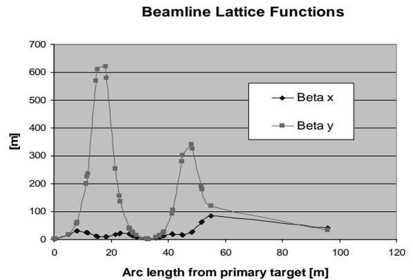
Figure 2. Beamline lattice functions: beam size is determined using an emittance of  $3-5\pi$  mm-mr.
