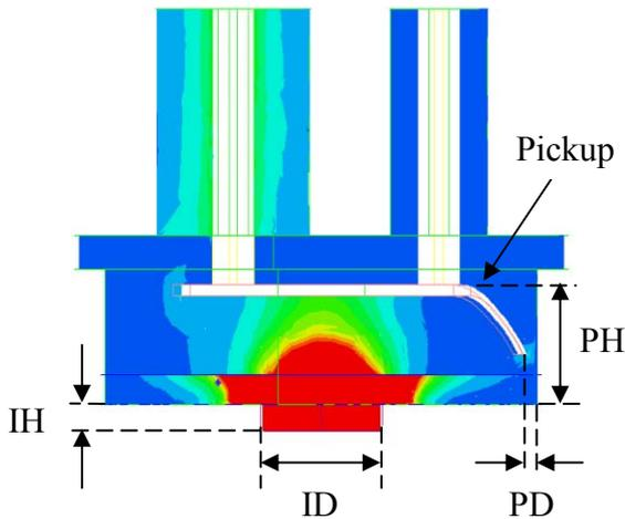
Figure 3: Electric field magnitude in coupler element. Parameters associated with the simulations and measurements are defined as follows: PH: Pickup Height, PD: Pickup Distance, ID: Iris Diameter, IH: Iris Height.
