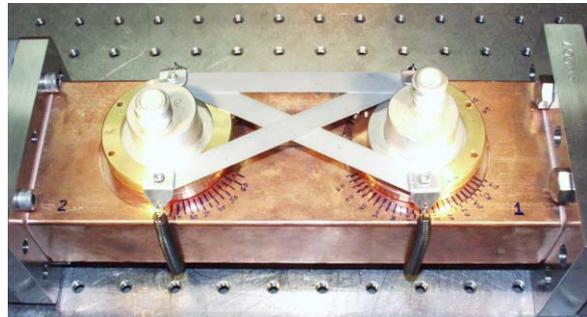
Figure 2: Coupler with spring assembly.
